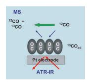
**Desorption and exchange of CO:** The exchange of a saturated 13CO adlayer by gas-phase <sup>12</sup>CO is monitored by in situ attenuated total reflection infrared spectroscopy (ATR-IR) spectroscopy and online mass spectrometry (see figure). First-order exchange and the dependence of the exchange rate on the partial pressure of <sup>12</sup>CO indicate CO<sub>ad</sub> desorption at room temperature and a desorption-controlled exchange mechanism.
